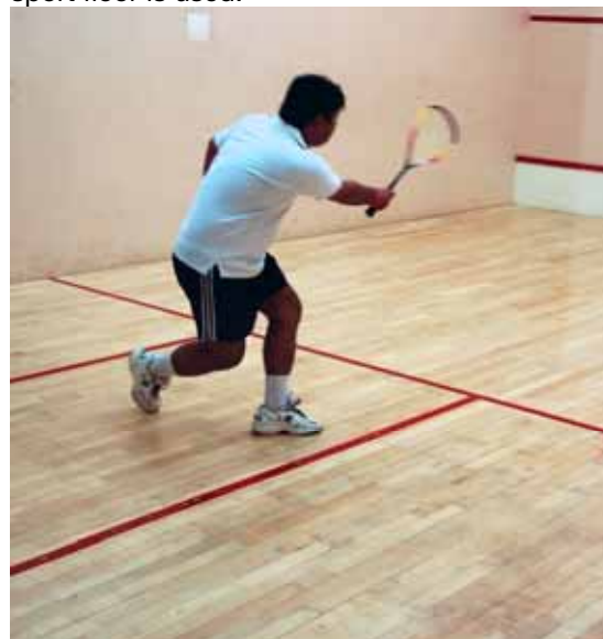
A typical squash court with a hardwood area elastic floor surface.
