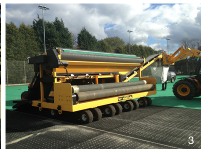
Automatic carpet lifting and rolling machine in operation
