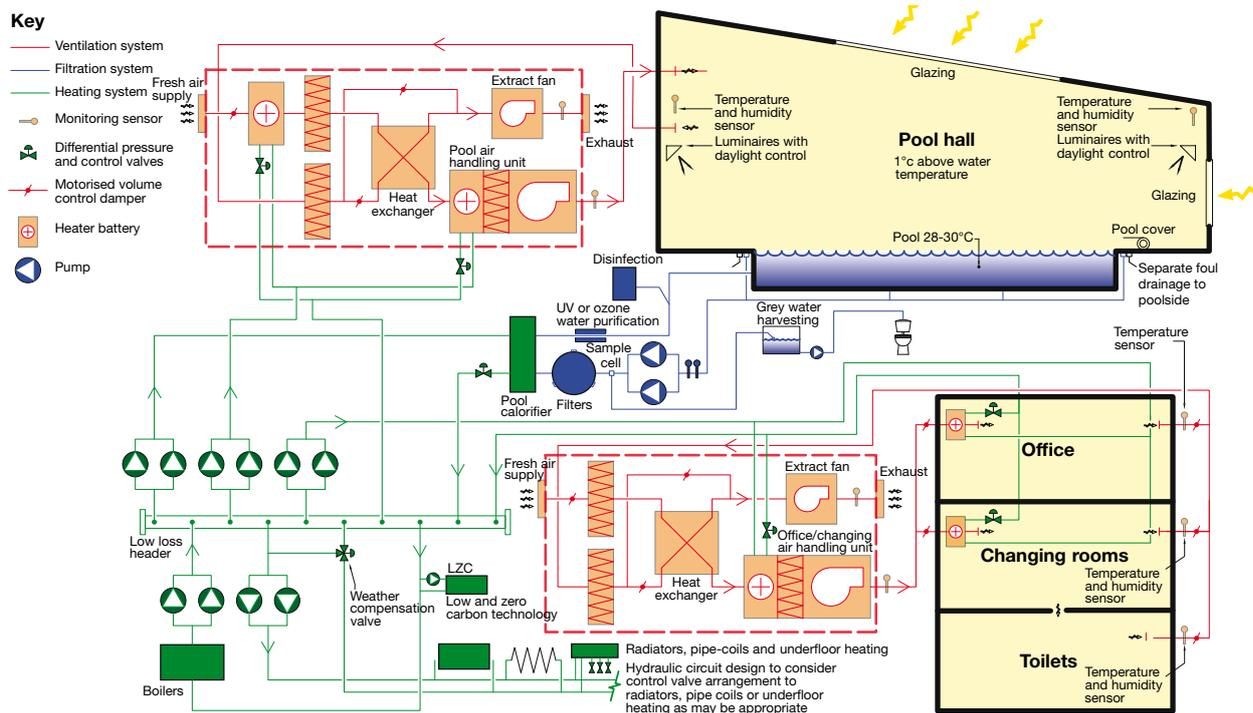
**Schematic services diagram for a typical small pool**
