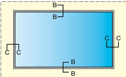
**Example plan of a general purpose swimming pool showing deck level edge channel provided to the perimeter of the pool tank. For competition use removable turning boards and starting platform can be used**
