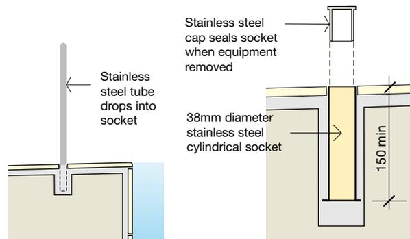
**'D' type socket - False start/backstroke warning poles**
