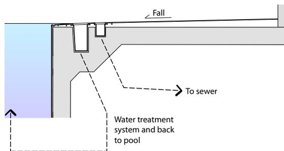
Example of pool channel drainage to meet BS EN 15288-1 : 2008
