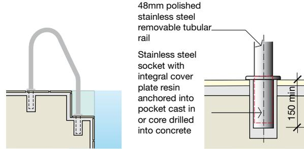
**'B' type socket - Pool entry step handrails**
